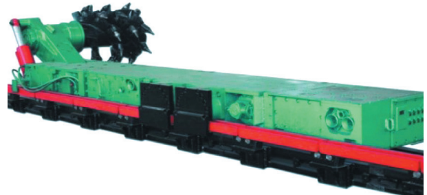
Fig. 9. HMG100/111-TWD one-head cutting shearer for thin seams produced by HOT
