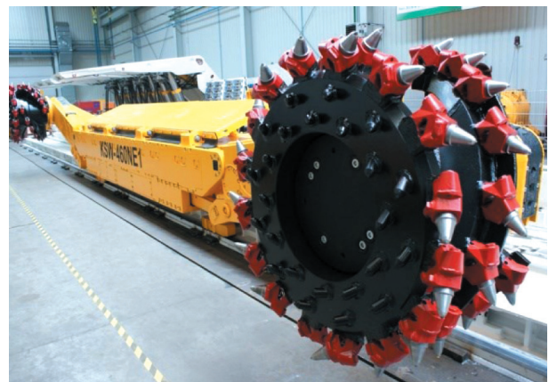
Fig. 3. KSW-460NE1 longwall shearer produced by Kopex Machinery
