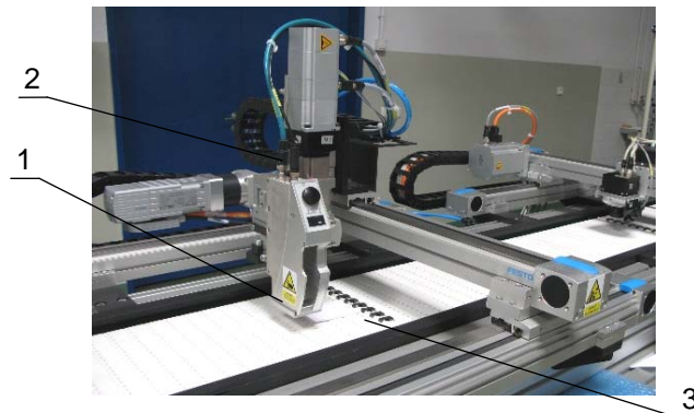
Fig. 5. Printing module: 1 – printing head, 2 – pneumatic actuator, 3 – clamps
