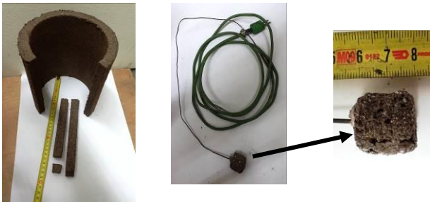
Fig. 7. Method of cutting a 20x20x20 mm specimen out of a sleeve and installation of a sheathed K thermocouple in its geometrical center
