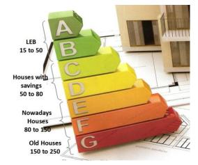
Fig. 2. Rating of houses by the specific heat consumption in kW·hour<sup>-1</sup>
