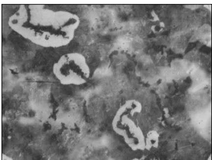
Fig. 5. Microstructure of test plate castings of vermicular cast iron; pearlite, traces of ferrite, vermicular graphite; digestion with 4% HNO 3 ; magnification 300x
