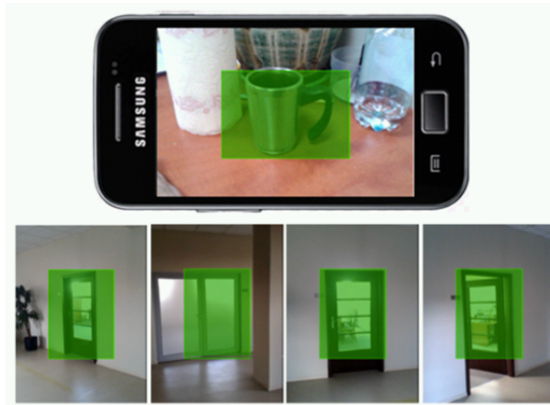
Fig. 8. Example of object detection (mug and doors) with proposed algorithm deployed on an Android device.
