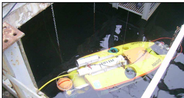
Fig. 2. Underwater vehicle MAGiS undergoing tests conducted by the Scientific Association ABYSAL in the Technological Pool of the Faculty.
