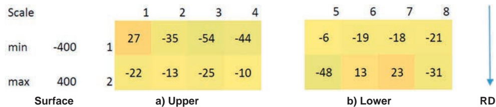
Fig. 5. Residual stress distribution of the upper (a) and lower (b) surface of the DC03 steel sheet before stretch levelling; RD – rolling direction
