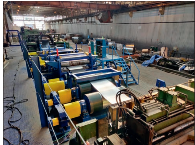
Fig. 1. Demonstration line with stretch leveller
