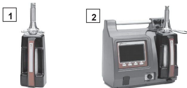
Fig. 1. Particulate matter analyzer ELPI+: 1 – impactor, 2 – general view [3]
