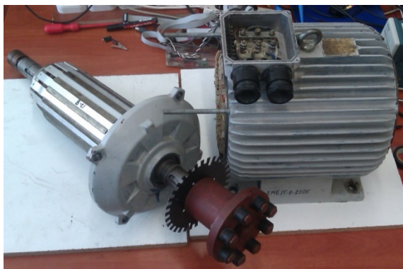
Fig. 7. View of a) measurement set, b) examined cylindrical synchronous generator
