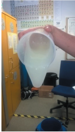
Fig. 4. Stable lip of crosslinked fracturing fluid (United Oilfield Services lab)
