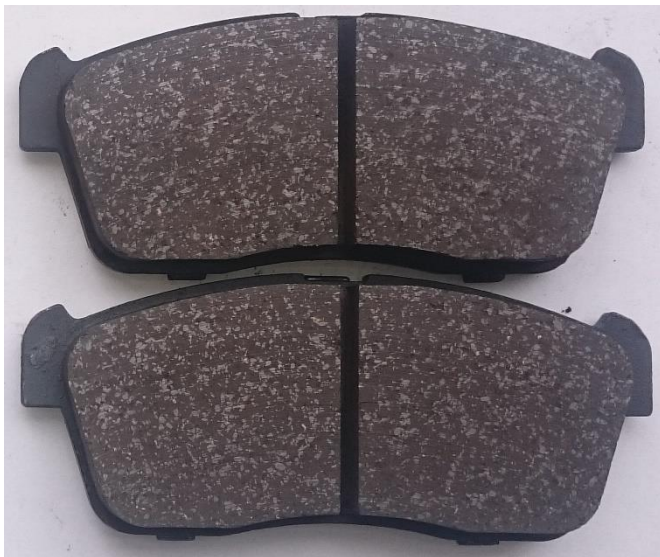
Picture. 4 The burnished brake pads – after the test.
