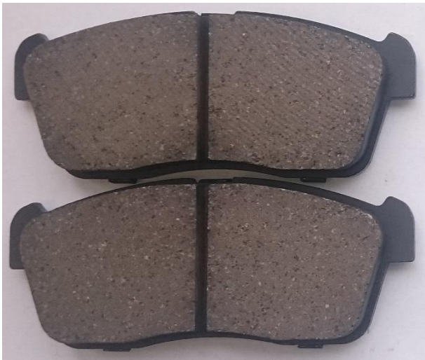
Picture 3. The unburnished brake pads before the test.
