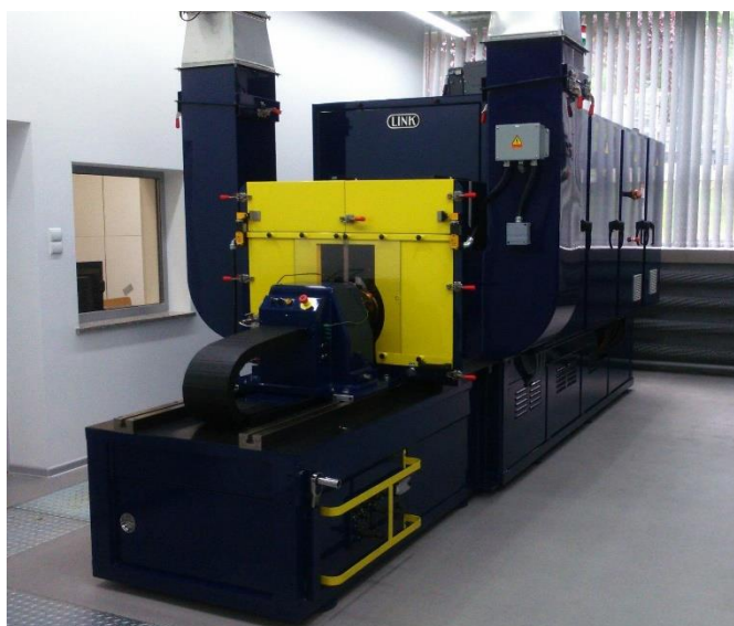
Picture. 2. The LINK M3000 Inertia Brake Dynamometer.
