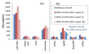
Fig. 7. NOx results for the on-road tests
