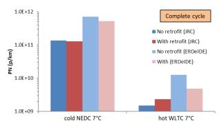
Fig. 4. PN results for the complete cycles
