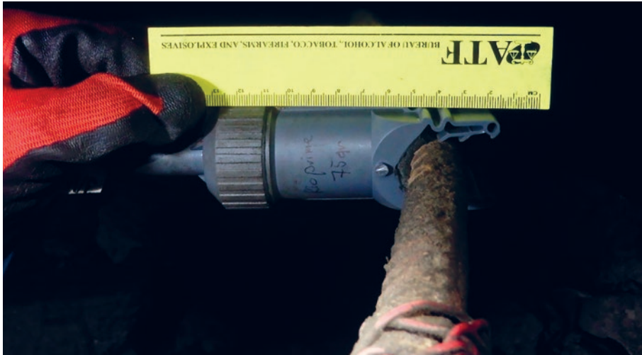
Fig. 11. ReBar Cutter™ fitting on a \varnothing 20 mm steel anchor Source: Private gallery (P. Hatys).
