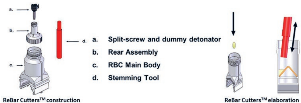
Fig. 12. Construction and method of ReBar Cutters™ elaboration Source: [9].
