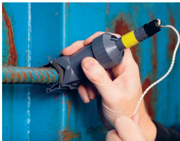
Fig. 9. Fitting the ReBar Cutter™ (RBC) on a steel bar
