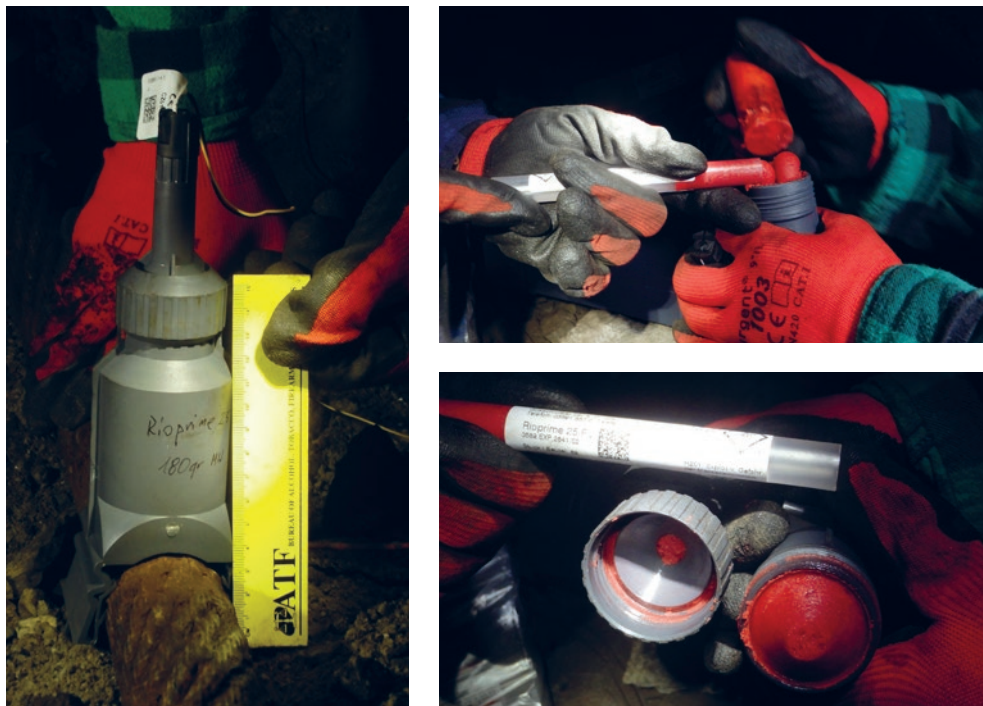
Fig. 15. 50 mm in diameter RBC charge attached to the still leveling cable \varnothing 55 mm filled plastic explosive RIOPRIME 25 weighting 180 gr Source: Private gallery (P. Hałys).
