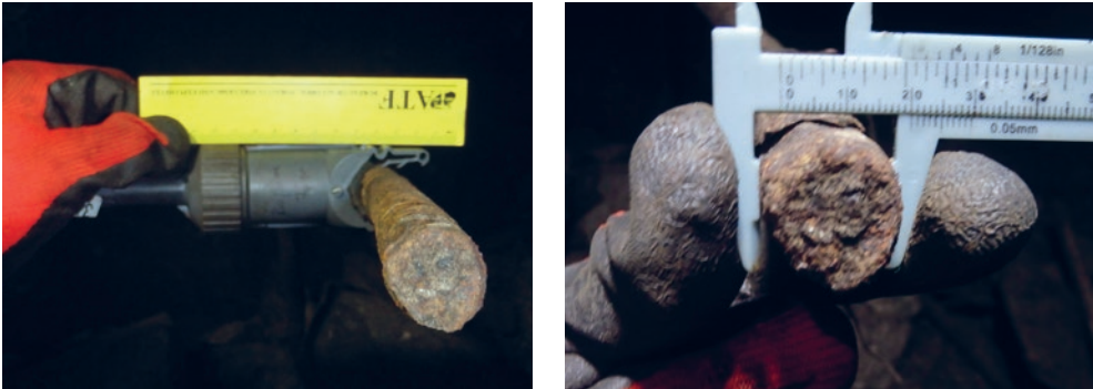
Fig. 17. 32 mm in diameter RBC charge attached to the still anchor rod \varnothing 20 mm filled plastic explosive RIOPRIME 25 weighting 75 gr Source: Private gallery (P. Hafys).
