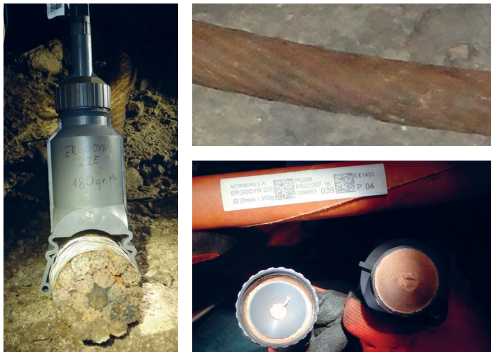
Fig. 13. 50 mm in diameter RBC charge attached to the still leveling cable \varnothing 55 mm filled rock blasting explosive ERGODYN 22E weighting 180 gr
