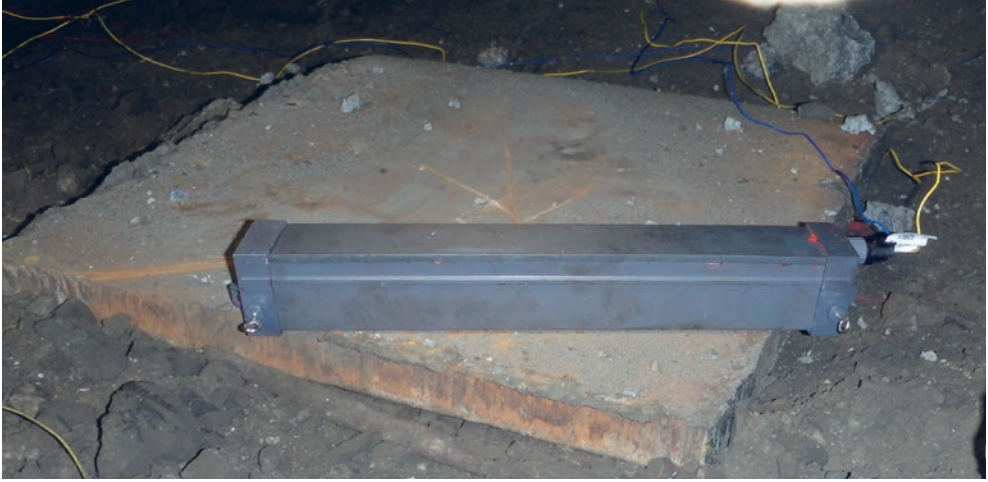
Fig. 24. 350 mm long DIOPLEX™ 400 charge attached to the element from bucket loader type LKP 903 40 mm thick filled plastic explosive RIOPRIME 25 weighting 140 gr Source: Private gallery (P. Hatys).
