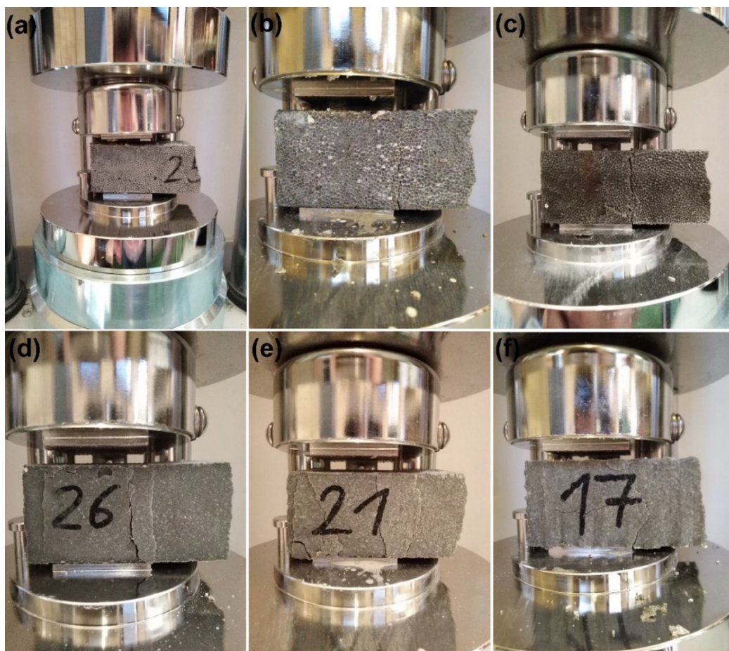
Fig. 9. Digital images obtained after compressive strength tests for reference sample (a) and samples with 0.5 wt.% admixture of Al 2 O 3 (b), lignin (c) and for samples containing 0.5 wt.% alumina-lignin hybrid materials 5:1 (d), 2:1 (e) and 1:1 (f)
