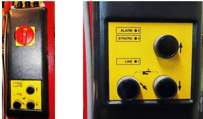
Fig. 19 Standard control panel that operates the lift.
