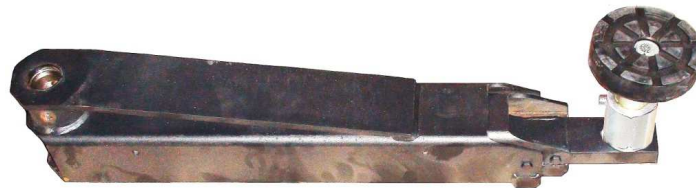
Fig. 4 Standard arm mounted to the lifting unit of the lift (own photo).
