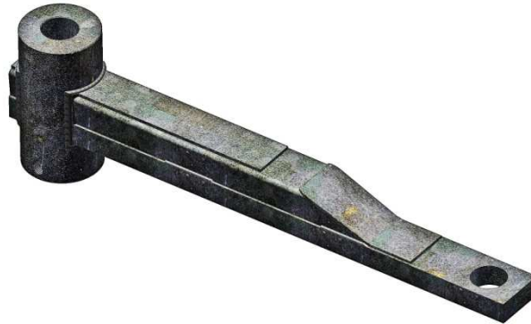
Fig. 6 The required arm structure for lifting the decompression chamber lid (study drawing by M. Palczewski-Haska).
