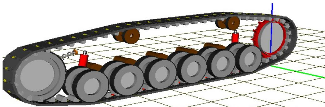
*Fig. 4. General view of modelled caterpillar mover*
