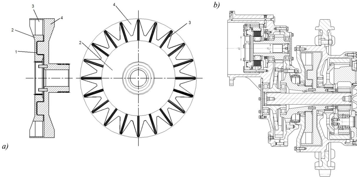
Fig. 1. a – elastic coupling construction; b – final drive unit with installed coupling
