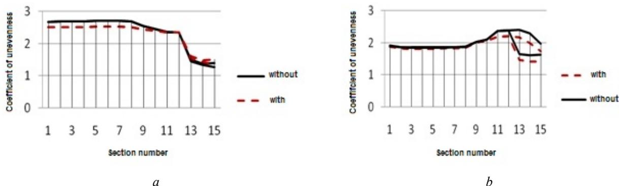
Fig. 10. Change of  $K_H$  on sections at exit from turn: a – speed is 2.78 m/s, turn radii is 2m; b – speed is 0.56 m/s, turn radii is 2 m
