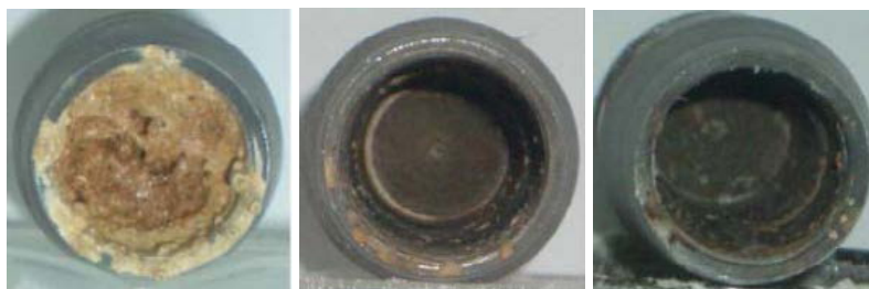
Figure 10. Removal efficiencies of TNT for the simulated warhead with a weight loading of 60 g of TNT at residence times of 5 min, 10 min and 20 min under the operating pressure and temperature conditions of 25 MPa and 55 °C
