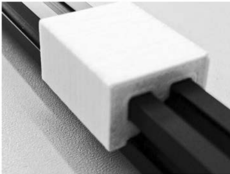
Fig. 2. Linear guideway block 3D-printed with Ibus filament [L. 4]
