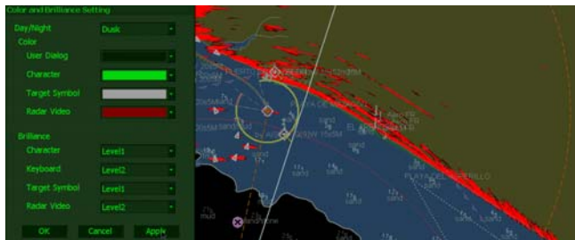
Figure 12. Radar overlay color pattern example on JRC ECDIS
