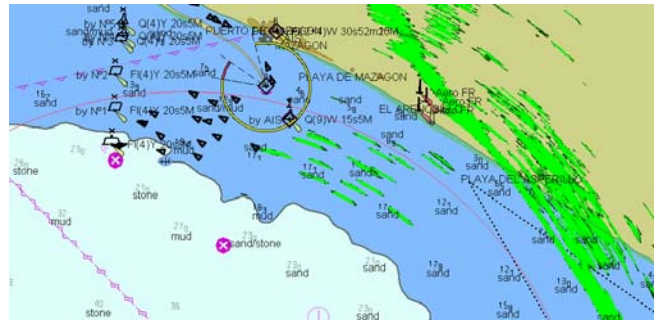
Figure 8. Radar Overlay not aligned with displayed chart
