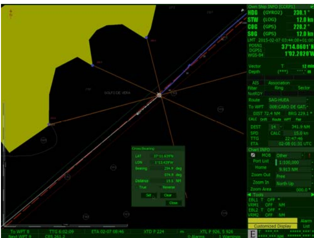
Figure 16. Observed position plotted by Cross Bearing function on JRC ECDIS
