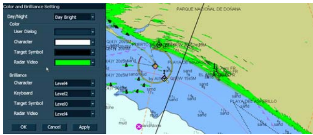
Figure 11. Radar overlay color pattern example on JRC ECDIS
