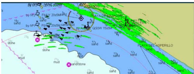
Figure 6. Radar Overlay not aligned with displayed chart
