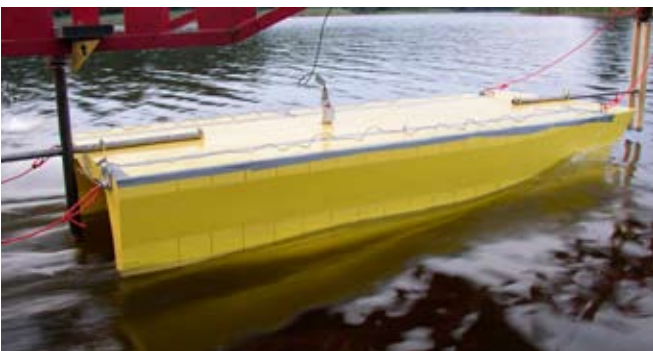
Fig. 21. Model of a SWATH catamaran during tests
