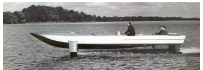
Fig. 7. The W-2 REKIN hydrofoil during tests on Jeziorak Lake.
