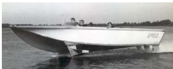
Fig. 9. The WS-6 hydrofoil during tests on Jeziorak Lake.
