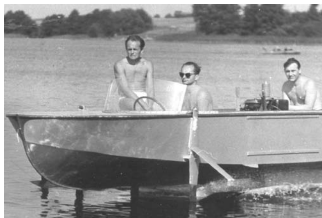
Fig. 2. Model of the K-2 hydrofoil during tests on Jeziorak Lake.
