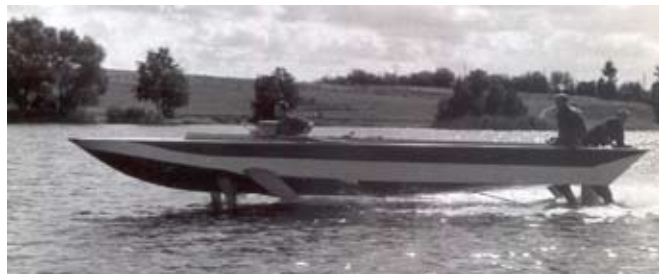
Fig. 8. The W-3 hydrofoil during tests on Jeziorak Lake.
