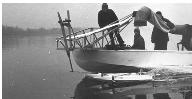
Fig. 11. The SP-04 hydrofoil model towed by SP-03 during tests on Jeziorak Lake.
