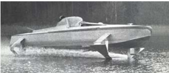
Fig. 4. The K-3 hydrofoil during tests on Jeziorak Lake.
