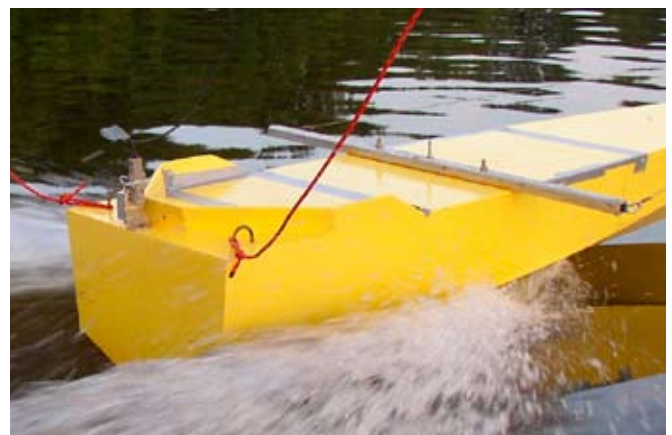
Fig. 18. No. 370 model in 1:16 scale during tests on Jeziorak Lake
