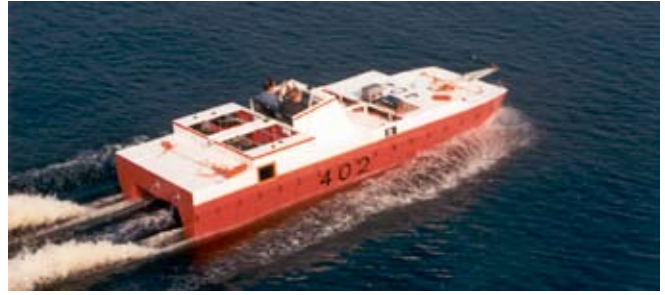
Fig. 22. Self-propelled model of a SWATH catamaran during tests on Jeziorak Lake
