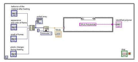
Fig. 2. Program view in block-diagram form
