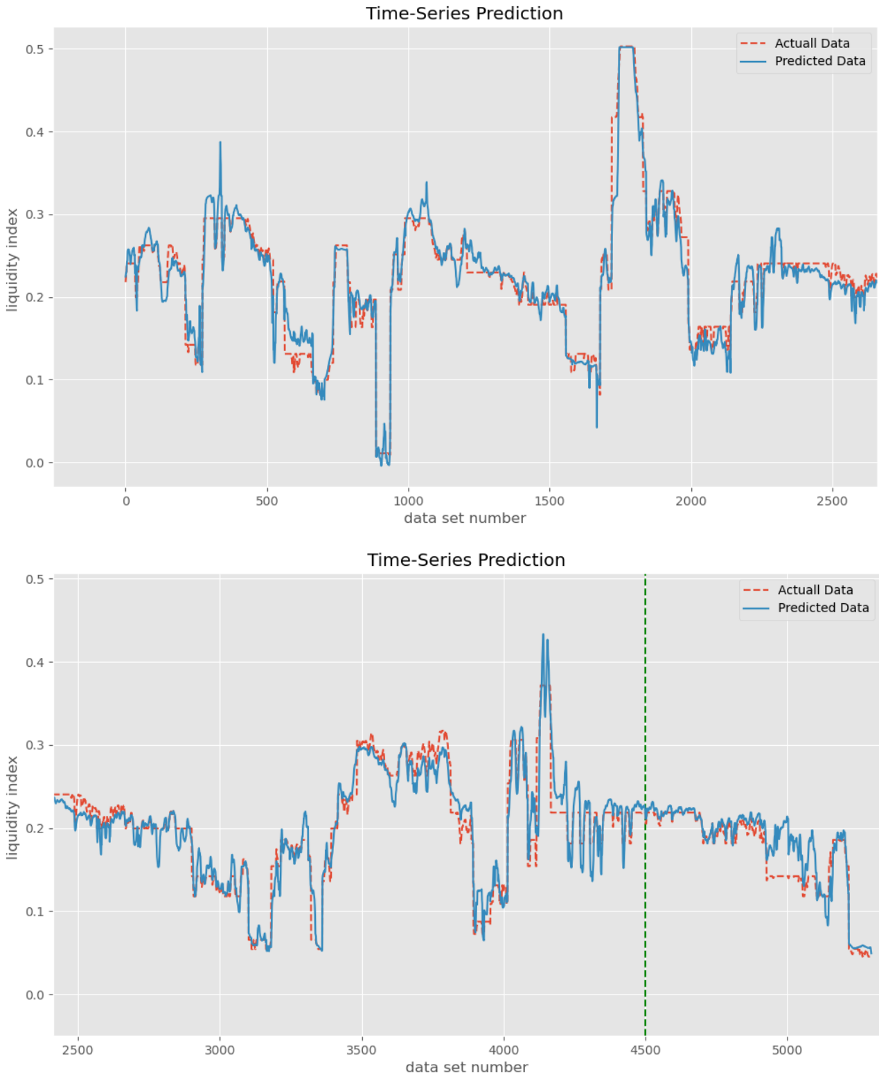
Figure 4: Results of identification of liquidity index with the developed LSTM network in comparison with known values of the liquidity index. Explanation in the text.
