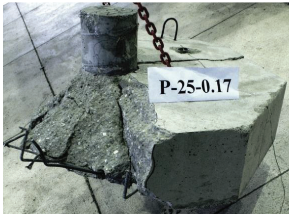
Fig. 11. Punching cone semi-exposed in P-25-0.17
