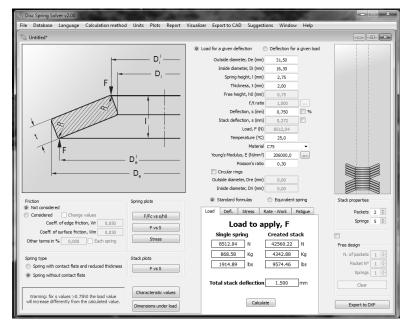
Fig. 5. Main window of Disk Spring Solver application [source: own study]
