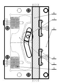
Fig . 4. Structure of skid catcher designed by LIFT Service S.A. [source: own study]
