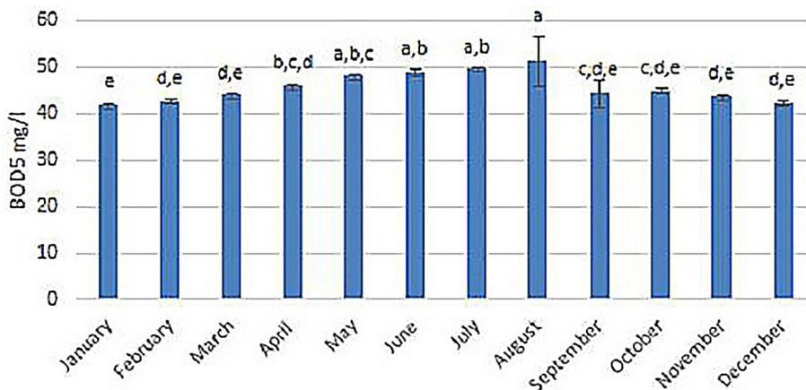
Figure 6. Biochemical Oxygen Demand (mean ± SD) for 12 months. Means that do not share the same letter are significantly different at p < 0.05
