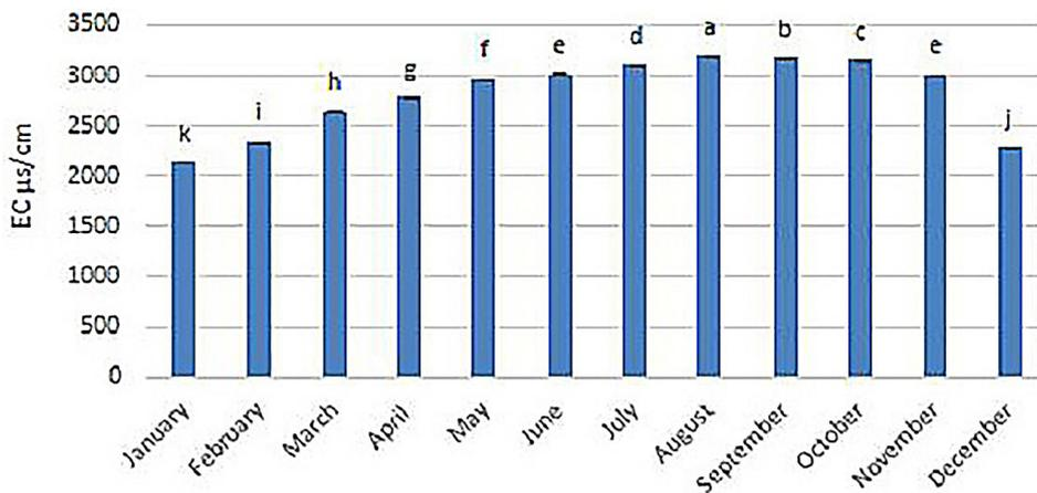
Figure 3. Conductivity variation (mean  $\pm$  SD) for 12 months. Means that do not share the same letter are significantly different at  $p < 0.05$
