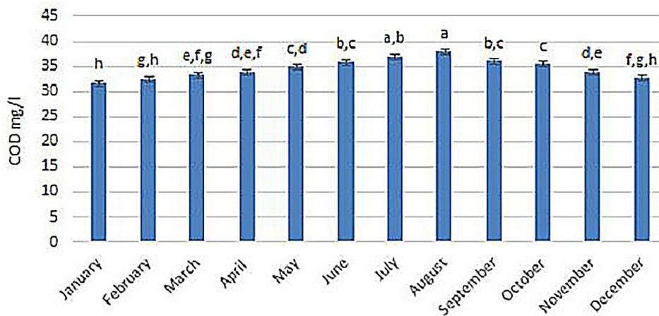
Figure 5. Chemical oxygen demand (mean ± SD) for 12 months. Means that do not share the same letter are significantly different at p < 0.05
