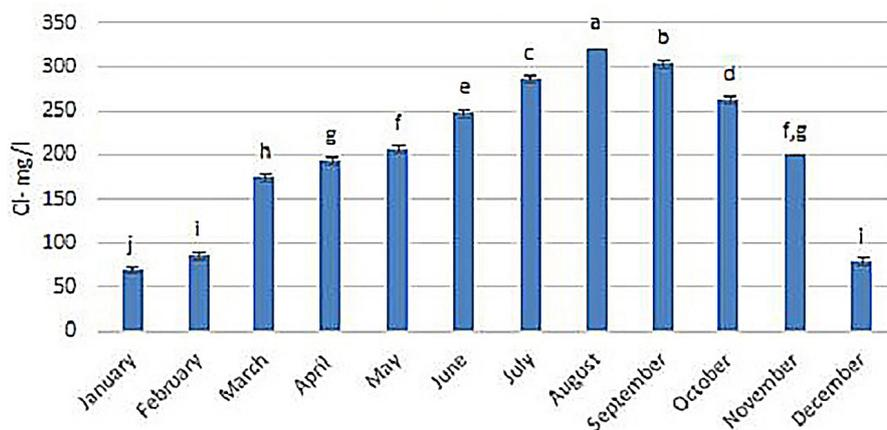
Figure 10. Chlorides (mean ± SD) for 12 months. Means that do not share the same letter are significantly different at  $p < 0.05$
