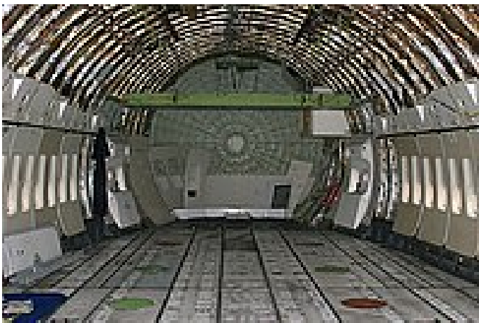
Fig. 6. View of rear bulkhead in L1011 wide-body plane reinforced by stringers and rings on internal passenger side
