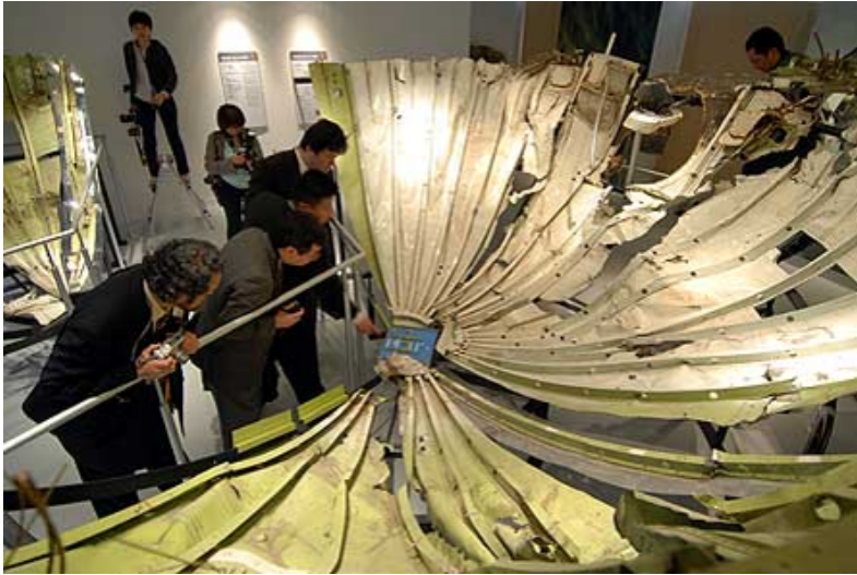
Fig. 7. Fragments of recovered rear bulkhead of JAL B747 plane in Tokyo airport museum
