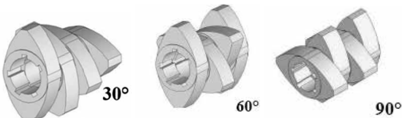
Figure 2. Kneading elements of a twin screw extruder.
