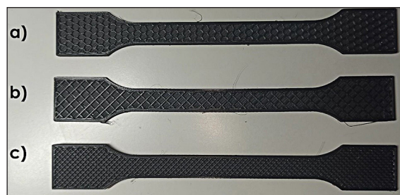
Figure 1. Types of sample filling (30% filling, view for 60% of the print) a) honeycomb, b) grid, c) line
