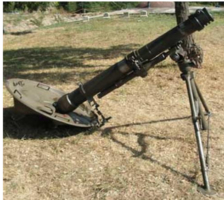
Fig. 3. Mortar, 120 mm M-120 model 43, with two visible grooves on the tube intended for mounting the clamping ring of the bipod at two different positions Source: Own collection
