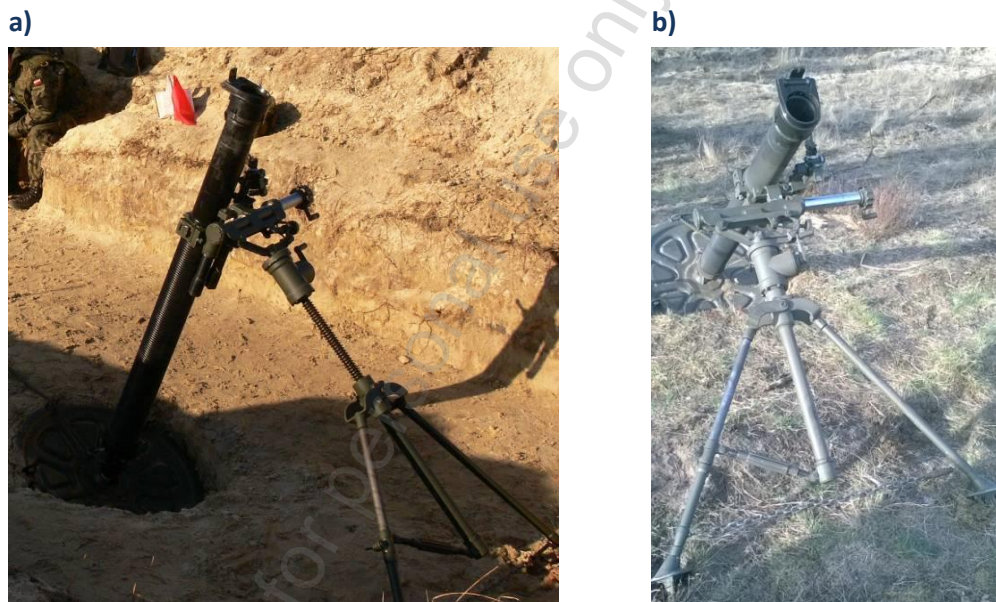
Fig. 4. a) M-98 mortar at the firing position with a high angle between the bipod and the tube with the extended worm gear of the elevation mechanism b) M-98 mortar at the firing position with the unstable positioning of the bipod spurs in relation to the ground surface. Source: Own collection
