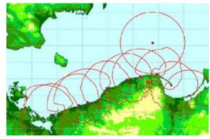
Figure 2. Areas monitored by the Polish network of the shore-based AIS stations after its modernisation and expansion (Urząd Morski w Gdyni, 2015)
