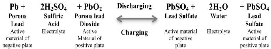
Fig. 6. Electrochemical Reaction of Lead acid battery [10]
