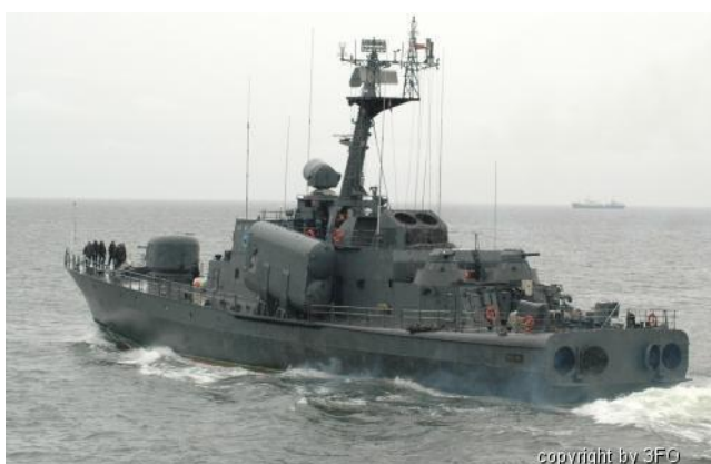
Fig. 1. 1241 RE missile corvette ( D = 490 t, v = 45 w; D — displacement, v — speed of ship) [42]
