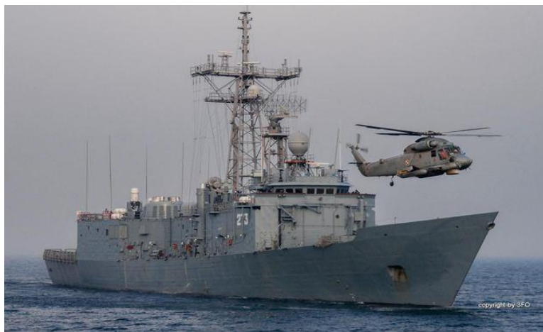
Fig. 3. 'Oliver Hazard Perry' type missile frigate ( D = 3\,600\text{ t} , v = 29\text{ w} ; D — displacement, v — speed of ship) [42]
