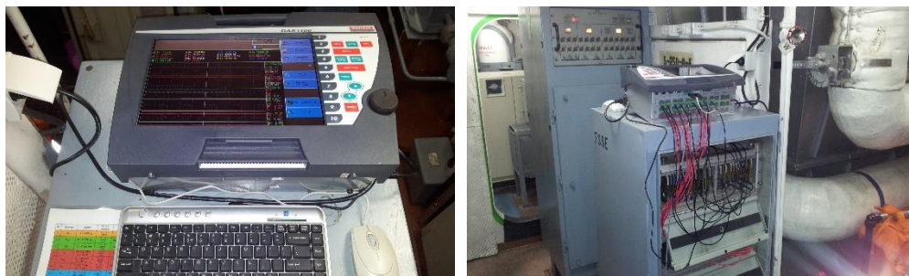
Fig. 17. The measuring and recording system Sefram DAS 1400 during energy research carried out on the ship [author's collection]
