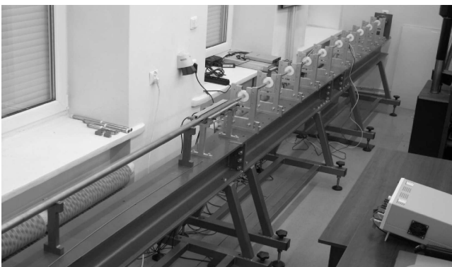
Fig. 1. Split Hopkinson Pressure Bar used in investigations
