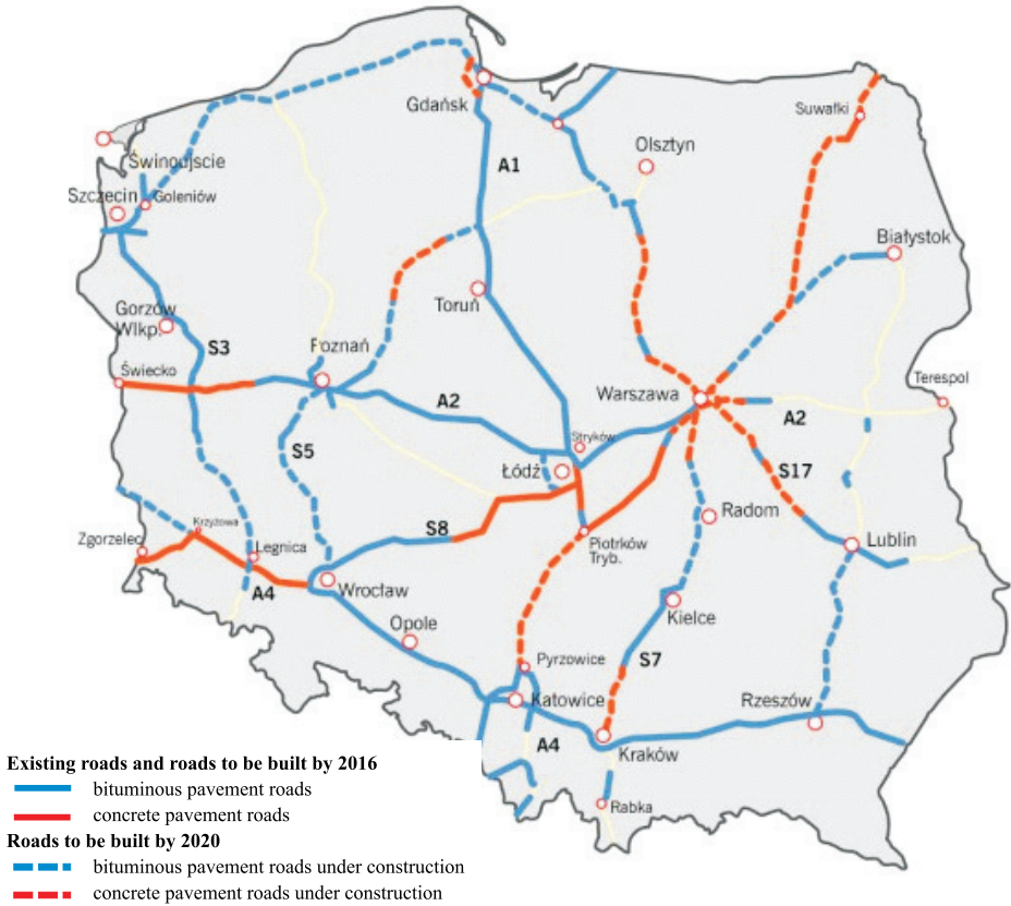
Fig. 1. Proposed types of pavements for the network of Polish expressways to be built by 2020, according to the General Directorate for National Roads and Motorways [7]
