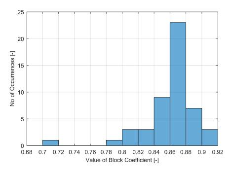
Figure 1 Distribution of block coefficient in Great Lakes bulk carriers. Based on data in [13]
