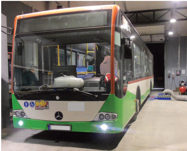
Fig. 1. Research object at the chassis dynamometer
