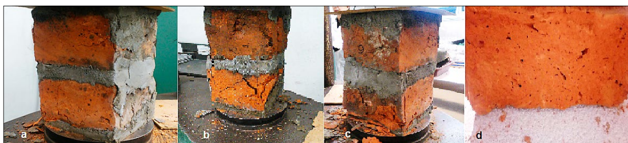
Fig. 3. Bricks in a material strength testing machine – determining strength through compression (a–c), brick porosity (d); photo by Ł. Bednarz.
