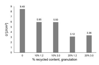
Figure 4. Impact of recyclate content % and granulation on impact resistance [J/cm<sup>2</sup>]
