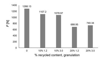
Figure 6. The effect of recyclate % and sieve on force  $(F_{max})$
