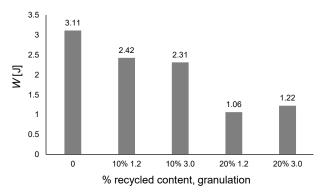
Figure 5. The effect of recyclate content % and granulation on energy (W)
