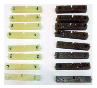
Figure 1. Charpy impact test specimens
