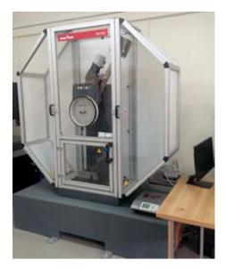
Figure 2. Swinging hammer, model RKP450 from Zwick Roell
