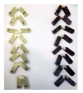
Figure 3. Samples after Charpy impact test
