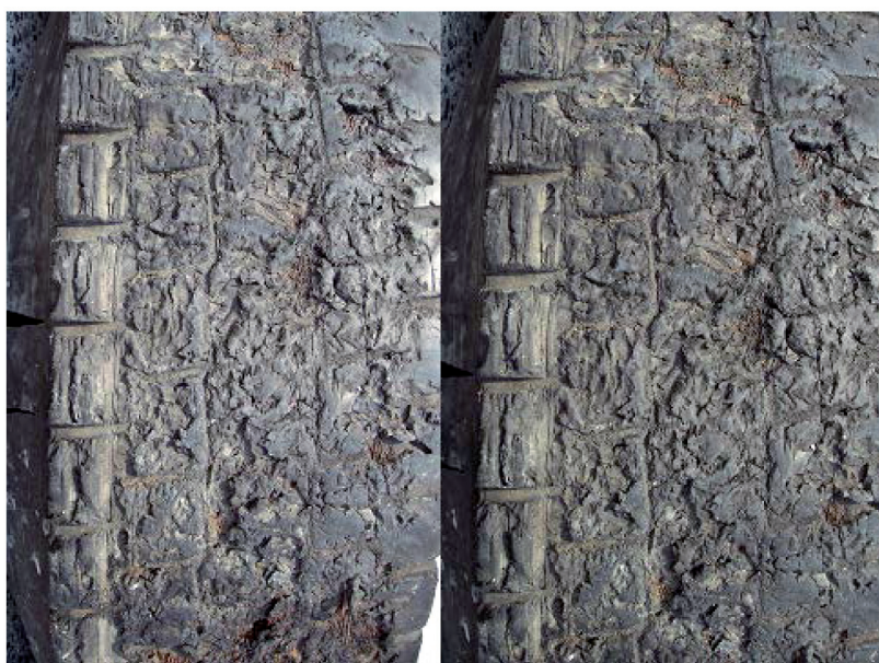
Fig. 2. Wear of tires – Chip-Chunk effect
