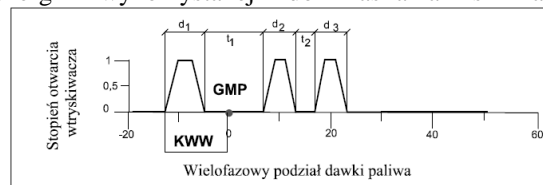
Fig. 2. Scheme of multiple injection of pilot dose Diesel oil
