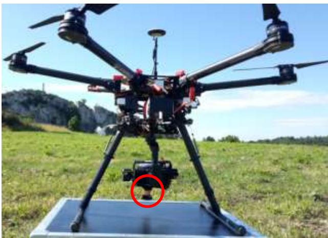
Fig. 1. Location and installation method of the Mini360 prism on the UAV
