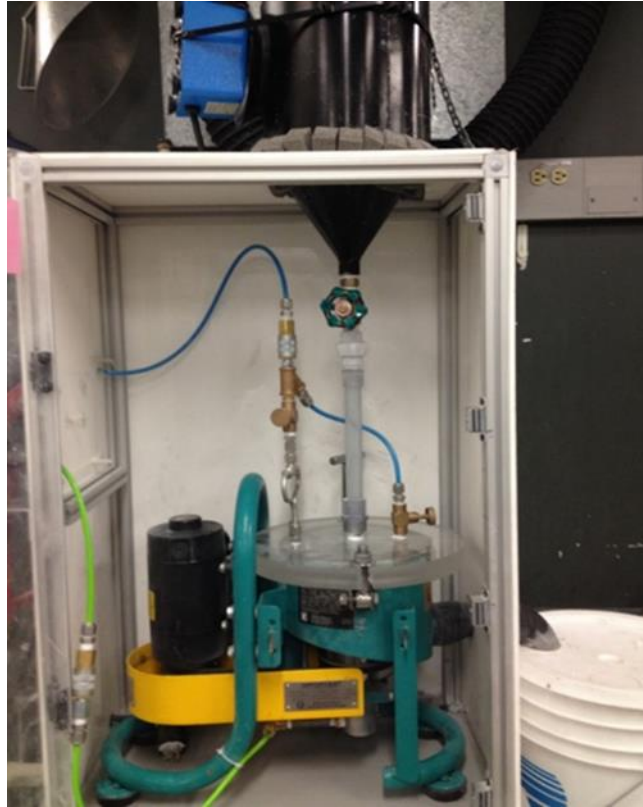
Fig. 2. Modified dry laboratory Knelson Concentrator
