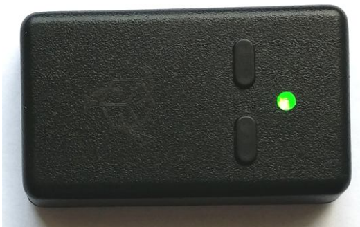
Fig. 3. YEI 3-Space sensor (features: 2 input buttons and RGB indicator)
