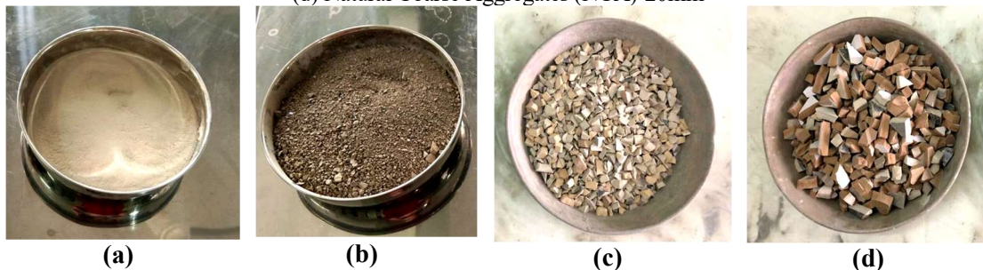
Fig. 2. (a) waste ceramic cement ( C_{WC} )-75 \mu m (b) waste ceramic sand ( S_{WC} )-4.75mm (c) waste ceramic aggregate ( A_{WC} )10mm (d) waste ceramic aggregate ( A_{WC} )-20mm
