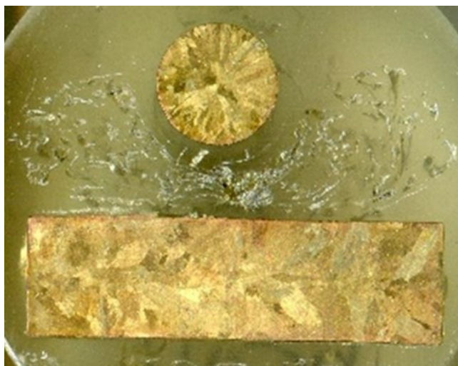
Fig. 9. Structure of CuZn39Pb2 castings - cast 8 (x1.5)
