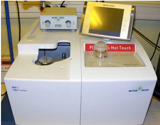
Fig. 1. Differential scanning calorimeter Mettler Toledo DSC 1
