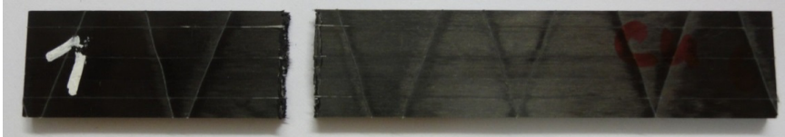
Figure 7. Rupture of a CFRP with copper after the bending test.
