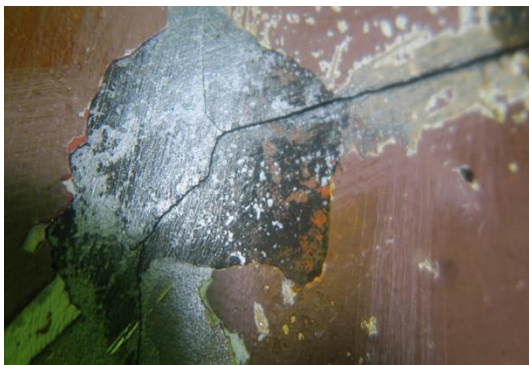
Figure 2. Crack in ship hull[10]
