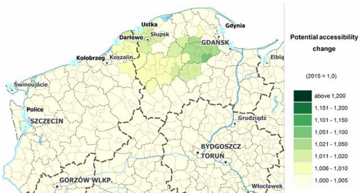
Ryc. 5. Improvement of the potential accessibility due to the implementation of the new Tricity metropolis ring road. Source: Own elaboration, M. Stepniak
